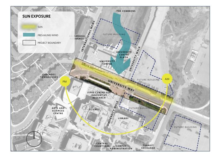
This diagram shows how the sun moves throughout the day. It shows that the majority of sunlight falls on the University Centre side of University Way. The diagram also shows the prevailing wind direction from the north.
